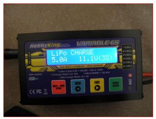
7. Then increase current to 5.0A and select 11.1V(3S).Hold start button to start charging. It will ask for confirmation. Then press start button again.
