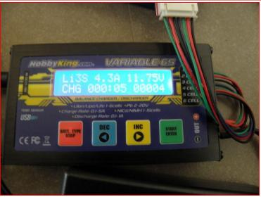
8. When charging is complete the charger will produce a beep sound. Disconnect the batteries .It will take 1hr to charge a completely drained battery.
