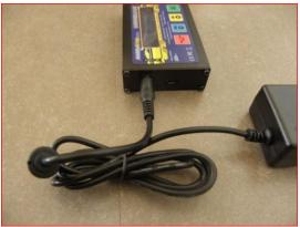
5. Now connect the balancer wire from the battery to balancer socket and crocodile pins from the charger to the battery terminals. NEVER INTERCHANGE THE TERMINALS.
